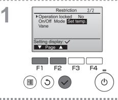
To enable the operation lock function, set the item "Operation locked" to " Yes".
